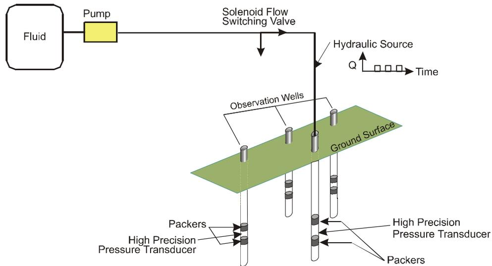
**FIGURE 1. Point Source Hydraulic Pulse Interference Test**
