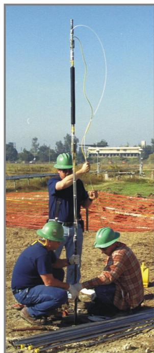
*Hydraulic Pulse Interference Test*
