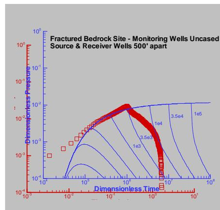
Type Curve Analysis of Pulse Test
