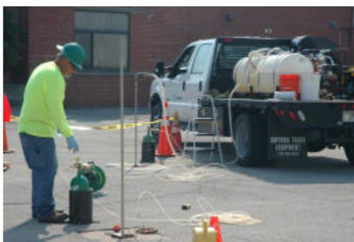
Pulse Interference Test Setup for Fractured Bedrock Site
