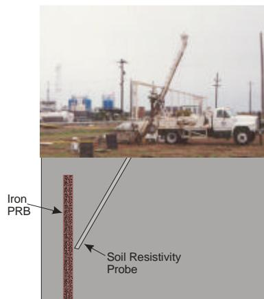
Inclined Profiling of PRB Thickness
