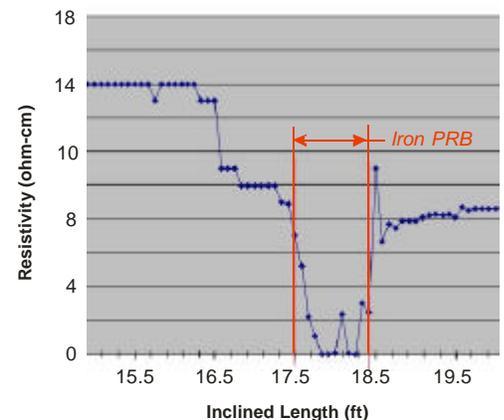
Soil Resistivity Profile for Determining PRB Thickness
