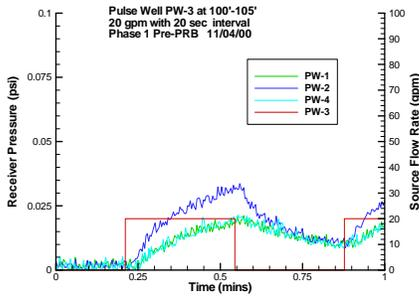
Hydraulic Pulse Interference Test Results
