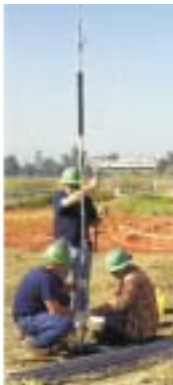
Typical Hydraulic Pulse Interference Test Setup
